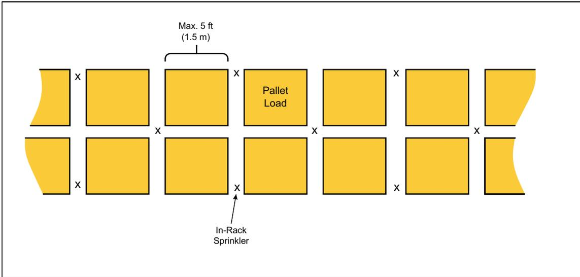
Fig. 2k. Horizontal in-rack sprinkler arrangement for open-top containers maintained in double-row racks having solid shelves greater than 64 ft<sup>2</sup> (6.0 m<sup>2</sup>) in area.
