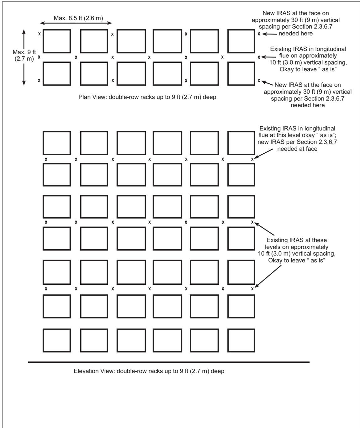
Fig. 24. Protection of uncartoned plastics in open-frame, double-row racks up to 9 ft (2.7 m) deep
