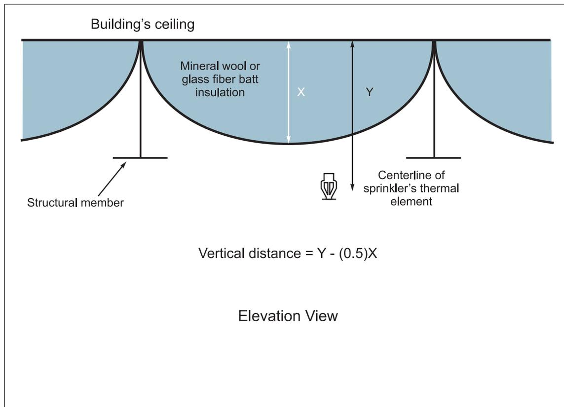
Fig. 25. Vertical distance between ceiling and centerline of sprinkler's thermal element in the presence of mineral wool or glass fiber batt insulation.
