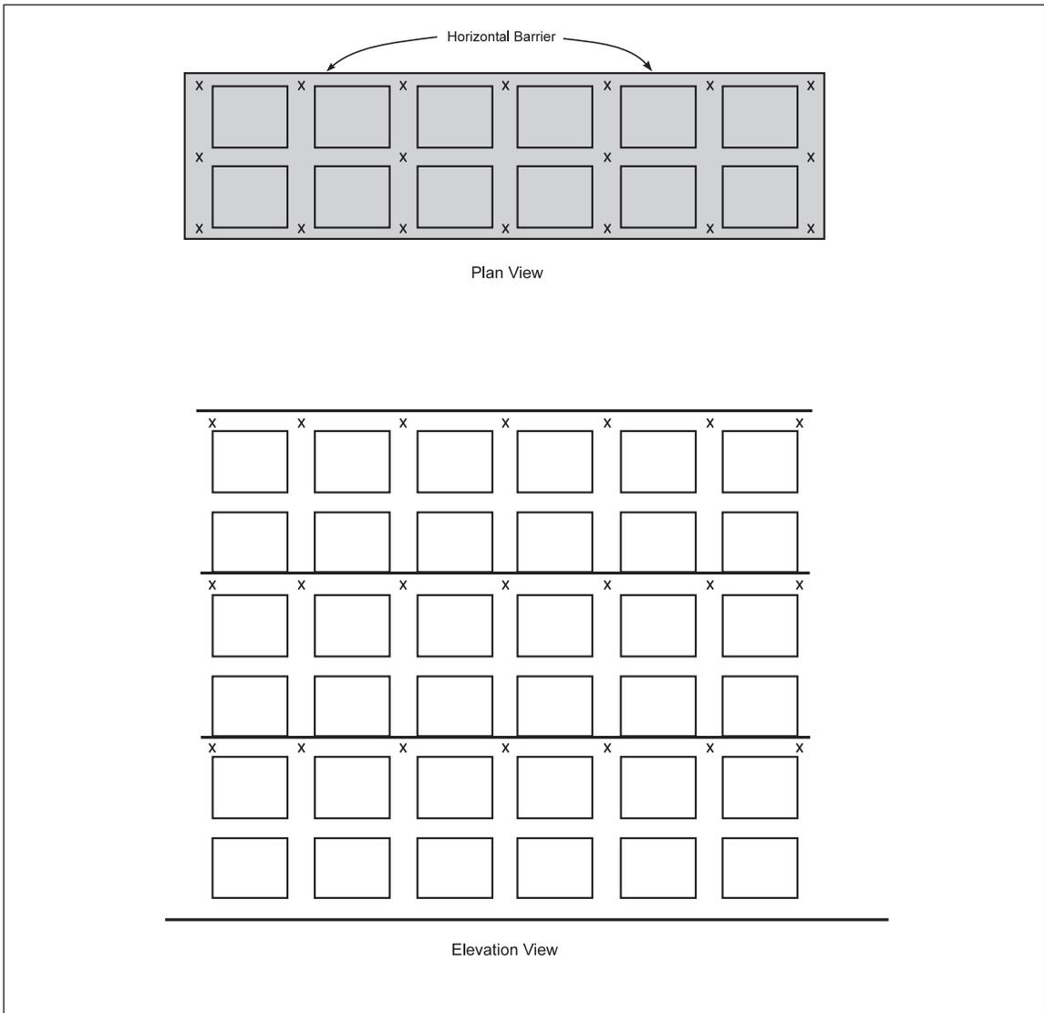
Fig. 17. Fire Protection Scheme 8-9A within double-row racks
